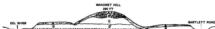
FIG. 92.—Diagrammatic section of Manomet Hill, Plymouth. A, glacial deposits; B, observed Truro deposits, 100 feet; C, supposed Truro deposits, 150 feet; D, sands and clays of unknown age, 100 feet; D', supposed continuation of D beneath the hill.
